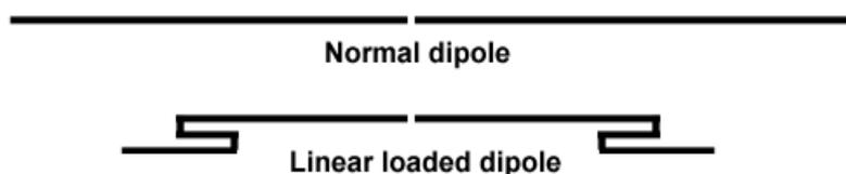
Picture 1 - Linear loaded dipole
